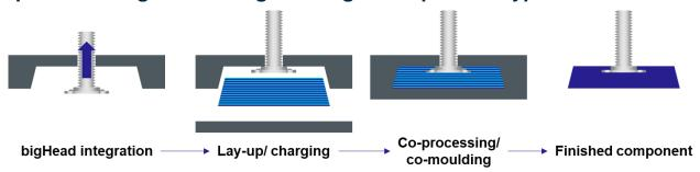
We refer to embedding as co-process integration; the embedded bigHead and the component materials are processed together within the principal manufacturing or forming process. This ensures the bigHeads are mechanically interlocked into the component material and eliminates the secondary operations associated with post-process fastener installation.
