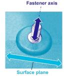
The terminology used to describe mechanical loading of embedded bigHeads may vary from other fasteners or fastening technologies
